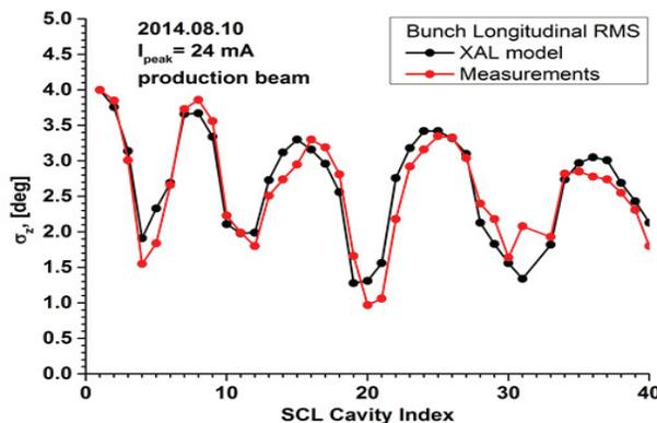
Figure 8: The RMS bunch length along the SCL. Measurements were performed by using the method described here.
