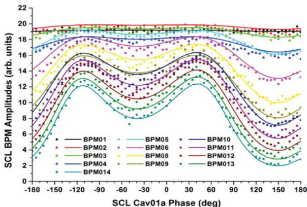
Figure 7: The BPM amplitudes during the first SCL cavity phase scan. Points are measurements; lines are from the envelope model.
