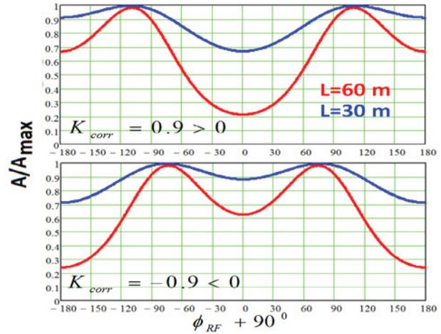
Figure 6: Amplitudes of BPMs at two distances for two cases of the phase-energy correlation
