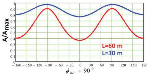
Figure 5: Amplitudes of BPMs at two distances as function of the synchronous phase of the first SCL cavity.
