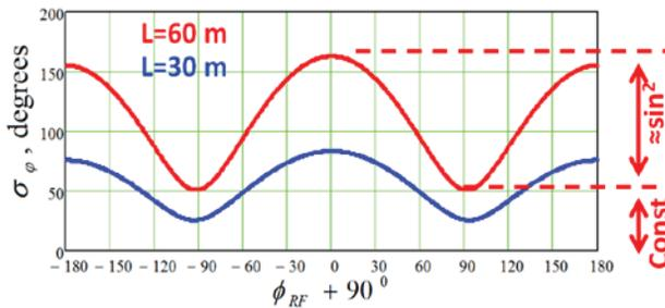
Figure 4: RMS longitudinal sizes of the bunch at two distances as function of the synchronous phase of the first SCL cavity.
