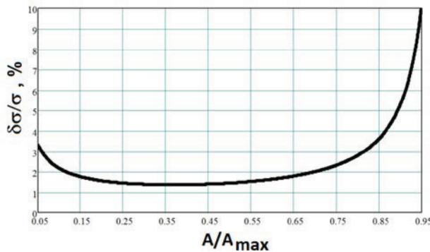
Figure 1: The relative error of bunch length measurements by using the formula (4). The BPM amplitude error is assumed 1%.
