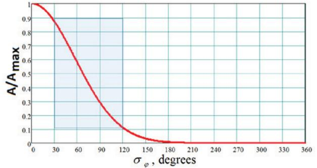
Figure 2: The range of measurable bunch lengths for the BPM's amplitude in 10%-90% range of the maximal value.
