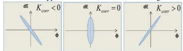
Figure 3: The longitudinal phase space for different types of phase-energy correlations.
