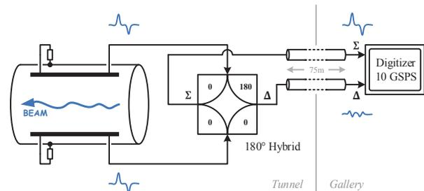
Figure 1: Block diagram of the LHC head-tail monitor.
