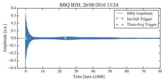
Figure 5: Comparison of the trigger algorithms during the transient caused by an injection.
