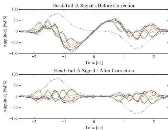
Figure 2: A mode  $|m| = 4$  instability, captured by the head-tail monitor, before and after the baseline removal.
