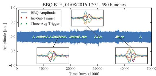
Figure 6: Instabilities with 590 nominal bunches that are seen by the three-averages algorithm but that would not be detected by the increasing-subsequence algorithm.
