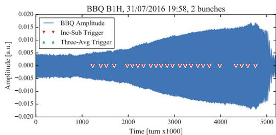
Figure 4: A slower instability, again with two nominal bunches, which is unseen by the three-averages algorithm but is detected by the increasing-subsequence algorithm.
