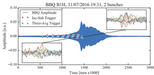
Figure 3: Comparison of the trigger algorithms during an instability with a two nominal bunches with markers indicating the trigger points of each algorithm. The inset plots show the head-tail monitor acquisition for the indicated triggers.
