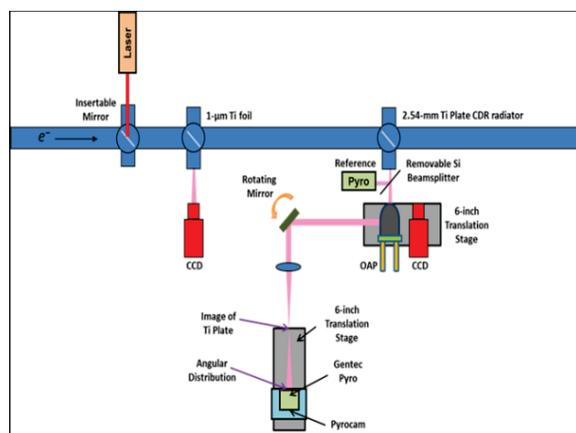
Figure 2: AD and PSF imaging system at FACET.
