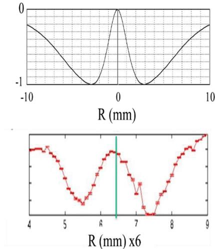
Figure 3: a) theoretical normalized horizontal line scan of the PSF of CDR from a flat rectangular radiator; b) measured normalized line scan of CDR distribution.
