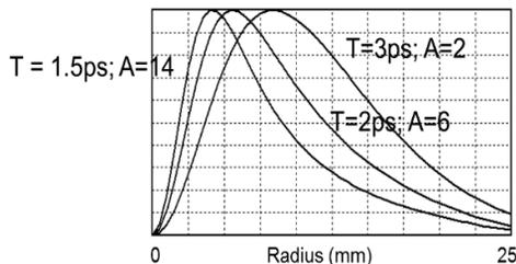
Figure 1: Theoretical CDR PSF distributions produced by a 100 MeV beam interacting with an annular radiator ( $R_{out}=25\text{mm}$ ,  $R_{in}=5\text{mm}$ ) for various bunch lengths.
