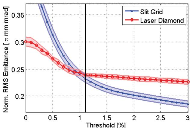
Figure 1: Normalized emittance resulting from both instruments as a function of threshold used for noise suppression.
