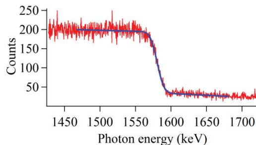
Figure 2: Measured CBS spectrum at 1.3 GeV with fit to determine the Compton edge energy.
